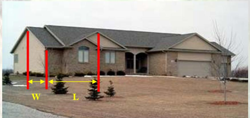
Example: This house has a simple roof. There is a gutter that collects the roof water from the peak and ridge on the front of the house. You would need to measure from gutter to peak which is "W" and from the end of the house to the ridge line which is "L". The drainage area is  $W \times L$ . Take your measurements in feet to get an answer in square feet.
